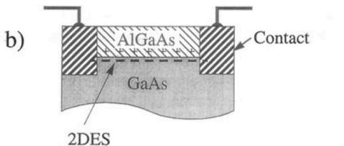
Observed in 2d electron systems, subjected to low temperatures and strong magnetic fields.
